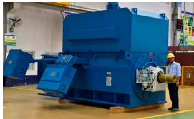
CG's 8.0 MW 6P 11kV Slip Ring Motor (one of the largest single drive cement mill motor in India)
