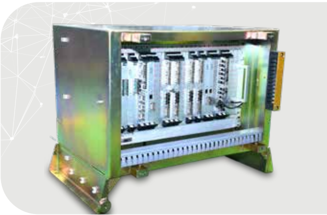
CG's TCN (Train Communication Network) based VCU (Vehicle Control Unit)
