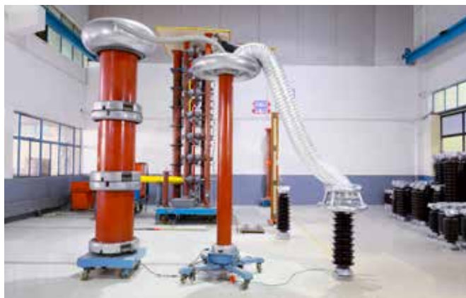
Surge Arrester under testing at CG's Nashik Testing Lab, Maharashtra, India
