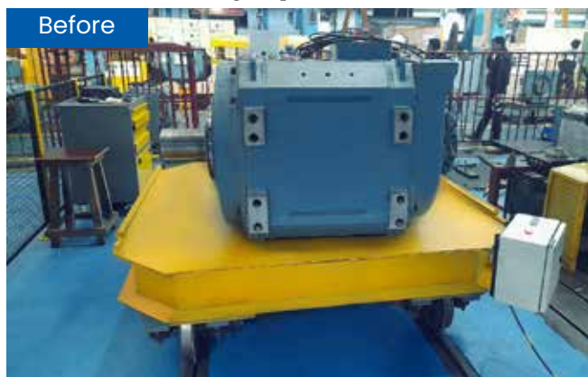
In this setup, there was no protective guard while conducting the manual operation on the above machine.
